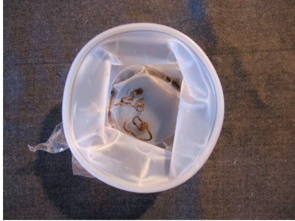
Figure #1: Photo micro-graph of the subject material submitted for evaluation. Basically this material appears to be “ribbons” of metal. The metal is Ferro-magnetic. Therefore it is most likely mild steel.
