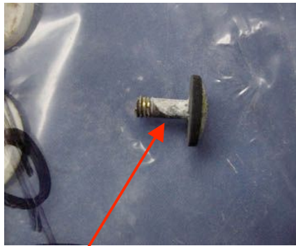
Figure #3: Photograph of what remains of the two hold down bolts. Both appear to have calcium deposits on them. This indicates that the holes were leaking.
