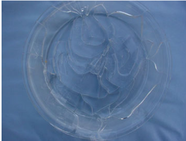
Figure #2: Photograph of the re-assembled dish. The failure origin is at the top of the photo. The "wandering" nature of the cracks leaving the origin indicates that the failure was driven by thermal stresses.
