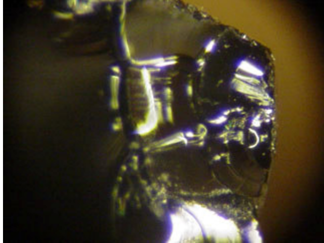
Figure #4: Higher magnification photo micrograph of a representative crush found at the failure origin (Mag 200X)
